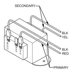
Fig. 5 – Transformer Connections
