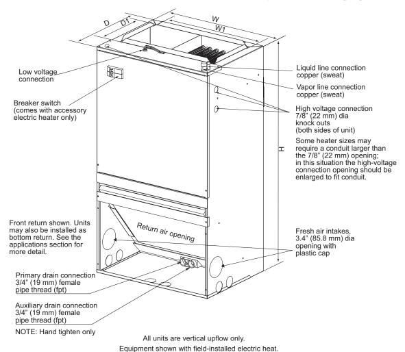
Fig. 2 – Dimensional Drawing with Circuit Breaker
