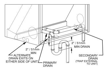
**NOTE:** Use plastic pipe from condensate pan to exterior of fan coil.
