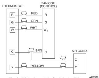
Fig. 6 – Wiring Layout Air Conditioning Unit (Cooling and 1-Stage Heat)
