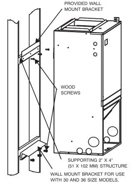
NOTE: Mounting wall and supporting structure must be able to support a minimum of 150 lbs. (68 kg)
