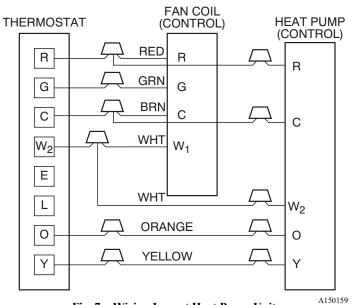
Fig. 7 – Wiring Layout Heat Pump Unit (Cooling and 2-Stage Heat)
