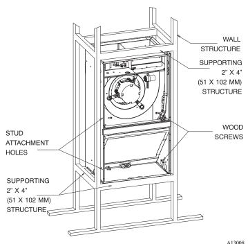
Fig. 4 – Frame Mount Installation
