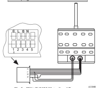
Fig. 8 – FMA4X ECM Motor Speed Taps
