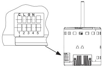
Speed Taps may be located on motor, or on plug close to motor.
