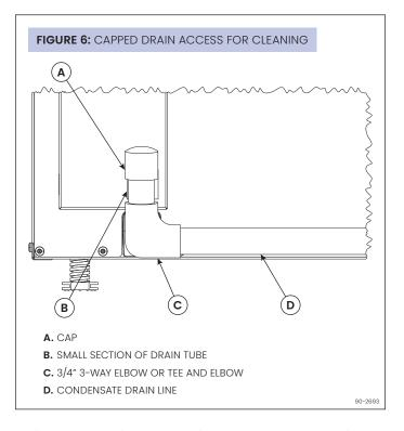
3. If the dehumidifier has clear flexible drain tubing, look for excess buildup in the drain line that might prevent water flow, and replace as needed. Clear, smooth, flexible 3/4" Inside Diameter (ID) drain tubing is available in most hardware stores or Do-It-Yourself (DIY) retail stores.
