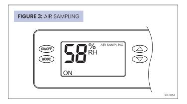
**4.** After sampling the air for 3 minutes, if the Relative Humidity (RH) is above the setting, the compressor turns on to dehumidify the space. **DEHUMIDIFYING** appears when the compressor is turned on (see **FIGURE 4**).
