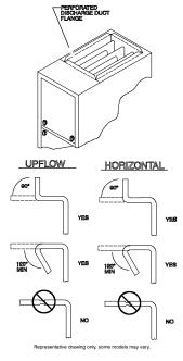
Fig. 20 - Duct Flanges
