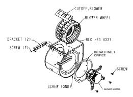
Fig. 66 - Blower Assembly on 040E14--10 and 060E14--12
