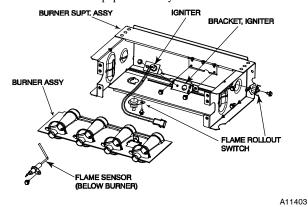
Fig. 68 - Burner Assembly
