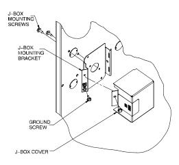
Fig. 35 - Installing J-Box (When Used)
