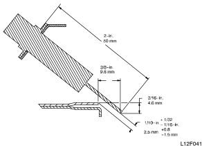
Fig. 70 - Igniter Position - Side View
