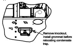
Fig. 18 - Horizontal Drain Trap Grommet INSTALLATION
