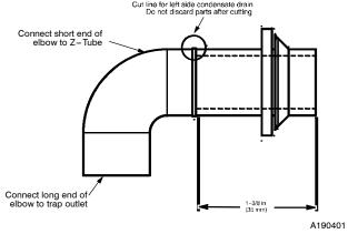
Fig. 17 - Modify Rubber Drain Elbow
