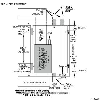
Fig. 6 - Air for Combustion, Ventilation, and Dilution for Outdoors
