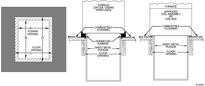
Fig. 25 - Installation on Combustible Flooring
