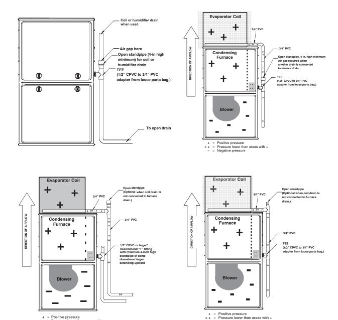
Fig. 12 - Example of Field Drain Attachment
