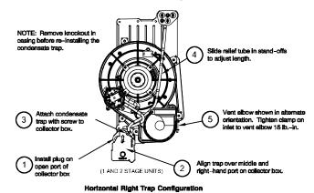
Fig. 10 - Horizontal Right Trap Configuration (Appearance may vary)
