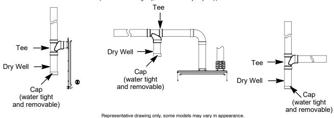
Fig. 51 - Recommended Combustion Air Inlet Moisture Trap
