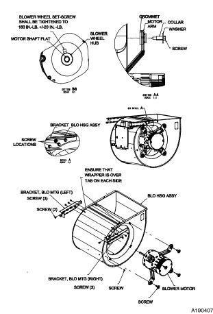
Fig. 67 - Blower Assembly on 100E21--22
