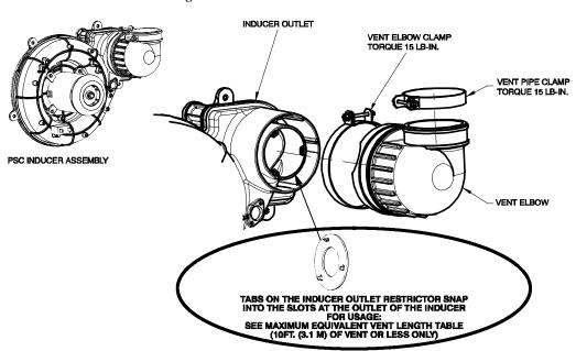
Fig. 53 - Inducer Vent Elbow
