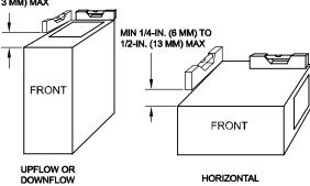
Fig. 19 - Furnace Pitch Requirements
