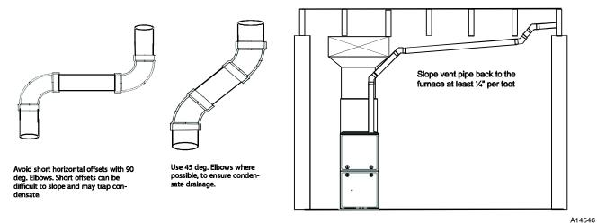
Fig. 52 - Near Furnace Vent Connections
