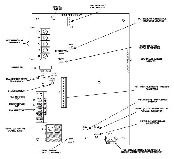
Fig. 37 - Example of Single Stage Furnace Control
