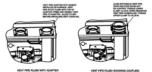
Fig. 59 - Optional Vent Pipe Flush with Adaptor
