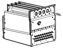
Fig. 71 - Cleaning Heat Exchanger Cell
