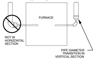
Fig. 50 - Combustion Air and Vent Pipe Diameter Transition Location and Elbow Configuration
