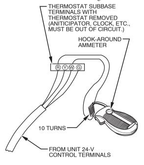
EXAMPLE:  $\frac{5.0 \text{ AMPS ON AMMETER}}{10 \text{ TURNS AROUND JAWS}} = \frac{0.5 \text{ AMPS FOR THERMOSTAT}}{\text{ANTICIPATOR SETTING}}$
