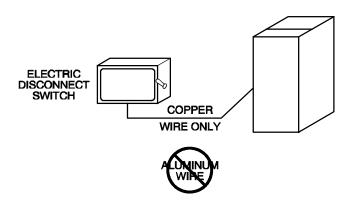
Fig. 34 - Field-Supplied External Electrical Box on Furnace Casing
