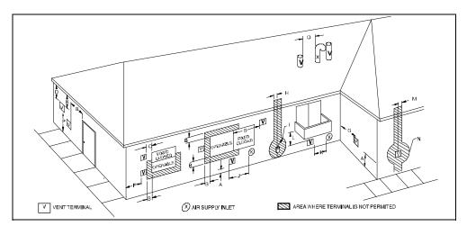
Fig. 42 - Direct Vent Termination Clearance
