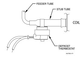
Fig. 3 – Defrost Thermostat Location
