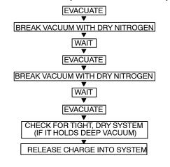
Fig. 15 - Triple Evacuation Method
