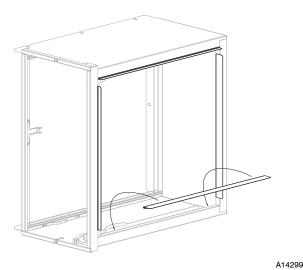
Fig. 6 - Use of Return Duct Adapters
