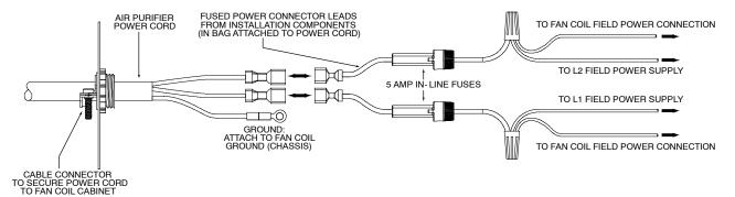
Fig. 10 - Fan Coil Chassis Ground
