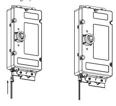
Fig. 7 - Airflow Sensor Cable Installed
