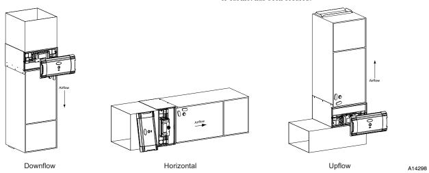
Fig. 4 - Infinity® Air Purifier Cabinet Orientation
