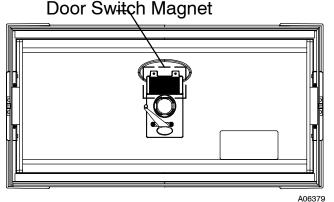
Fig. 13 - Door Switch Magnet
