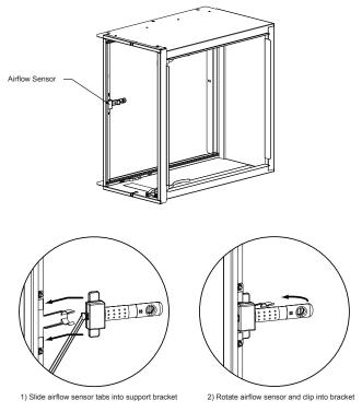
Fig. 12 - Airflow Sensor Install
