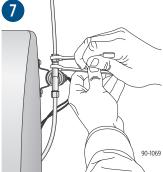
Tighten water line by double wrenching.
