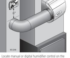
return 6" above the humidifier or bypass duct.
