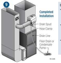
Drain Line: • Ensure downward slope and no kinks. • Do not overtighten hose clamp onto drain spud. • Do not use solvent adhesive on drain spud.
