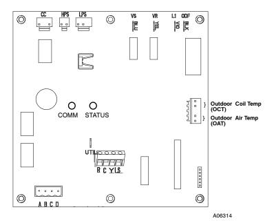
Fig. 10 - Single-Stage Control Board
