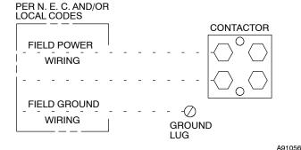
Fig. 5 - Line Power Connections
