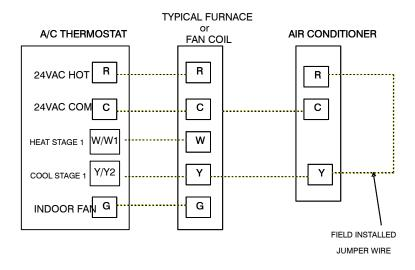
Fig. 13 - Non-Communicating Standard Thermostat 2-Wire 24V Circuit Connections (Applicable to units beginning with serial number 3006E and newer)
