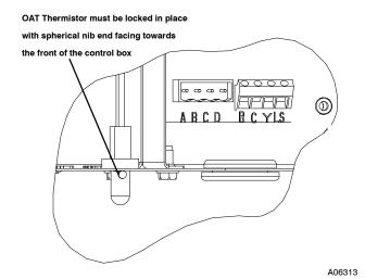
Fig. 6 - Outdoor Air Thermistor (OAT) Attachment
