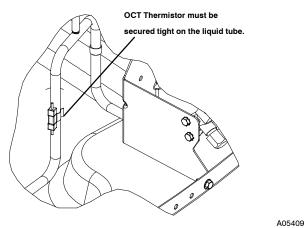
Fig. 7 - Outdoor Coil Thermistor (OCT) Attachment
