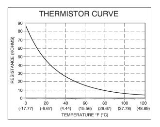
Fig. 9 - Resistance vs Temperature Chart
