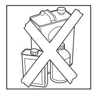
• Do not cover the furnace, store trash or debris near it, or in any way block the flow of fresh air to the unit.
