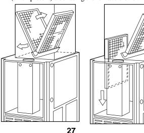
9. Replace blower door and secure with 2 screws. Turn on electrical supply to your furnace. (See Fig. 18.)
