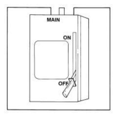
Fig. 3—Main Electrical Disconnect
