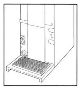
Fig. 4—Removing Filter from Fan Coil Unit
